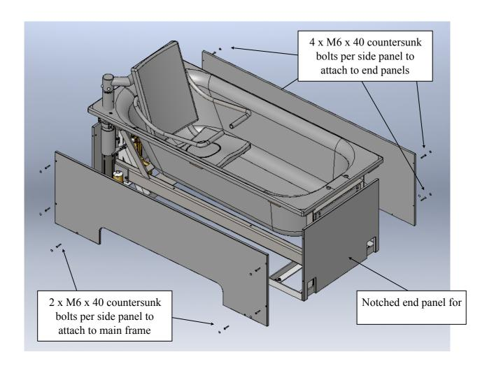
2. The side panels can now be attached to the end panels. These are secured with 4 M6 x 40 countersunk bolts per side panel, which screw into the threaded inserts located in the holes in the sides of the end panels. As these bolts are tightened ensure that the end of the front panel is flush with the face of the end panel, and that the top faces are also aligned. These are finished off with a white cap which pushes into the hexagon socket of the screw.
