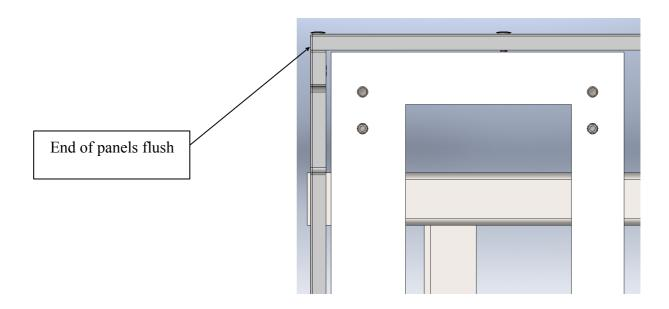
3. Once the panels are attached to each other (effectively creating a box around the bath), the complete inner panel assembly can be secured to the main framework using 4 M6 x 40 countersunk bolts (2 per side panel), which screw into the threaded holes on the bottom frame of the bath. As before, these are finished off with a white cap which pushes into the hexagon socket of the screw. There should be a gap of approximately 3mm between the bottom of the end panels and the floor.
