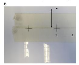
The dimension to the first hole can be 80mm from the top
